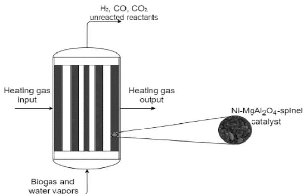
Fig. 1: Multi-tubular reactor with catalyst
