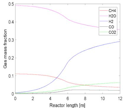
Fig. 2: Conversion of methane vs reactor length Fig. 3: Gas composition profile in multi-tubular reactor vs reactor length
