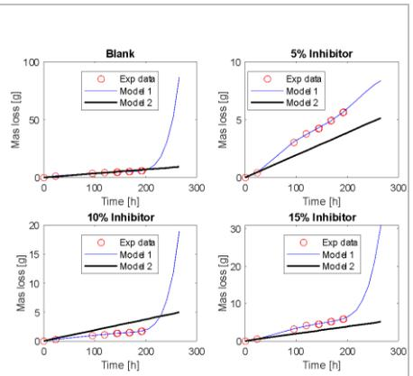
Figure 2 Compared results for the plate mass loss
