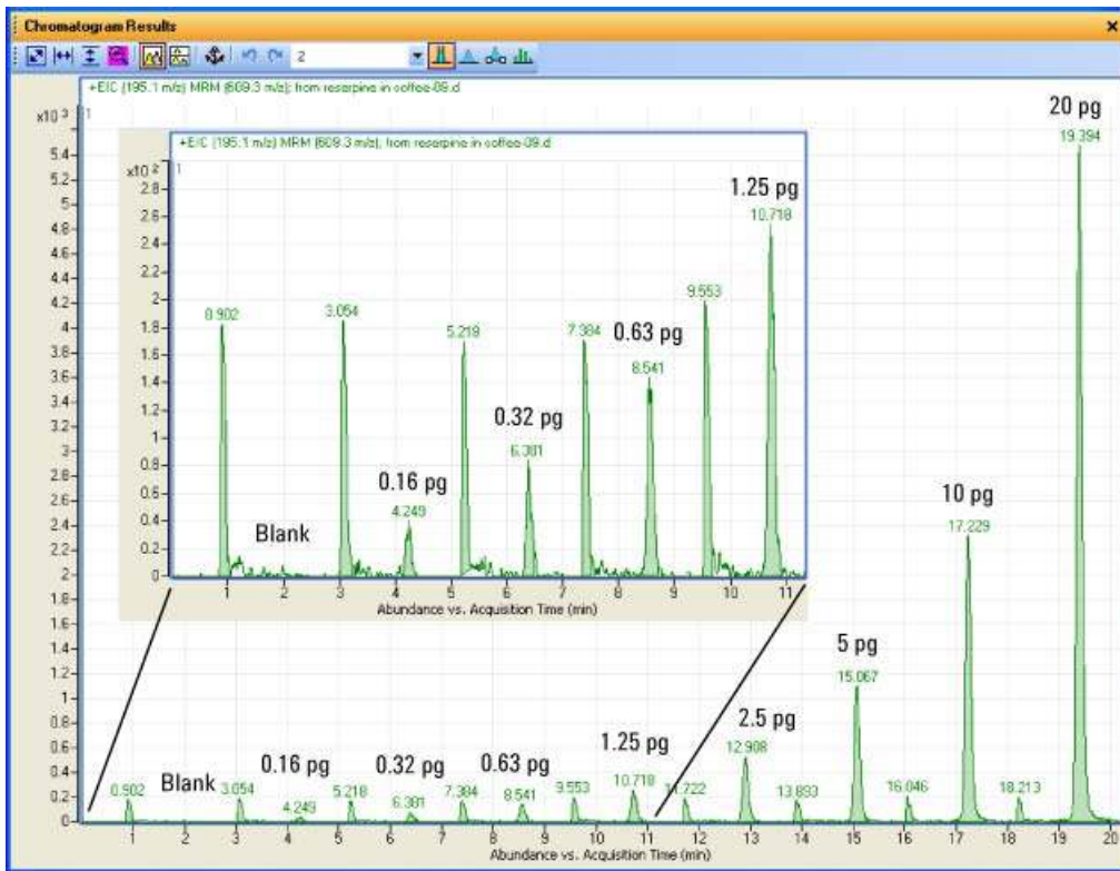
Figure 13 Reserpine Sensitivity for 6410 Triple Quadrupole (Specifications: 1 pg with S/N 50:1 or greater (3 x RMS noise))
