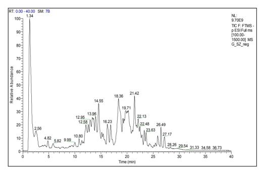
Figure 4. Total ion chromatogram of hydro-alcoholic extract of fenugreek in negative ionisation mode.
