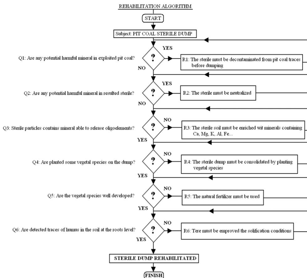
**Figure 1.** The sterile dump rehabilitation algorithm
