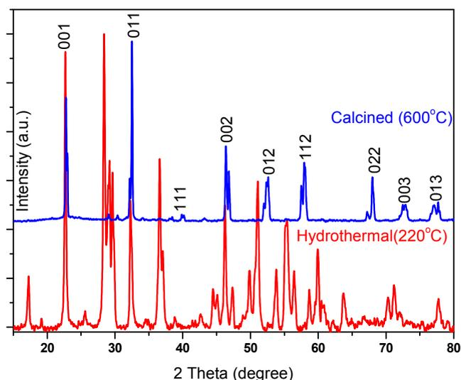
**Figure 1 a).** X-ray diffraction of  $\text{NaNbO}_3$  obtained by hydrothermal method at  $220^\circ\text{C}$  and after thermal treatment at  $600^\circ\text{C}$
