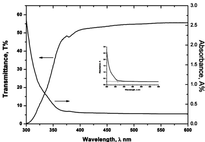
**Figure 6.** The absorption and transmission spectra of  $\text{NaNbO}_3$ , inset is represented the estimate band gap of  $\text{NaNbO}_3$ .
