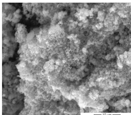
**Figure 2.** SEM images of mixed phases of  $\text{NaNbO}_3$  powder obtained by hydrothermal method at 220°C
