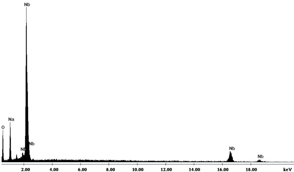
**Figure 4.** EDX images of single phase of  $\text{NaNbO}_3$  powder as obtained after the thermal treatment at  $600^\circ\text{C}$
