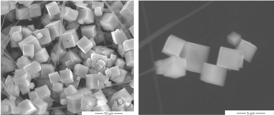
**Figure 3.** SEM images of single phase of  $\text{NaNbO}_3$  powder as obtained and thermal treatment at  $600^\circ\text{C}$
