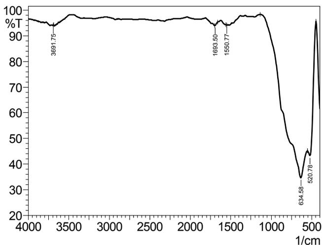
**Figure 7.** FT-IR spectra of the obtained  $\text{NaNbO}_3$  powder after thermal treatment
