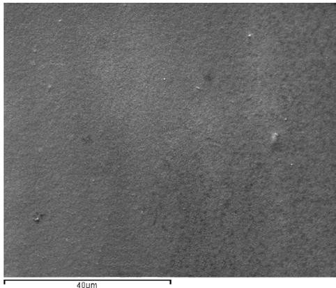
**Figure 1.** SEM micrograph of pure Zn deposits
