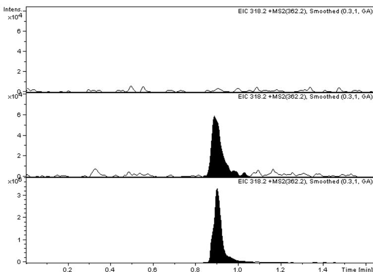
**Figure 2.** Representative chromatograms of (up) drug-free plasma, (middle) plasma spiked with levofloxacin at lower limit of quantification (0.1 µg/mL) and (down) plasma sample obtained from a patient 4 h after administration of 500 mg levofloxacin in perfusion (concentration found: 4.18 µg/mL).
