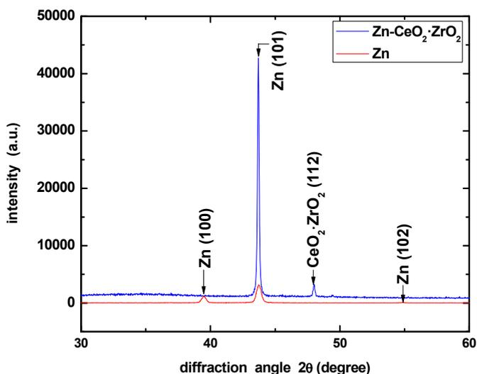
**Figure 3.** X-ray Diffraction results for the Zn and Zn– $\text{CeO}_2\text{-ZrO}_2$  deposits,  $1.25 \text{ g L}^{-1}$
