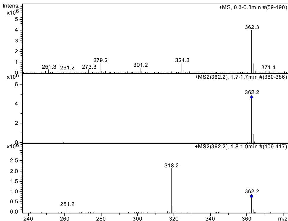
**Figure 3.** Mass spectra of levofloxacin obtained by electrospray ionisation in positive ion mode at the collision energy of 1.2V: (up) full-scan spectrum; (middle) MS spectrum of pseudo-molecular ion  $[M+H]^+$ ; (down) MS/MS reactive spectrum (after fragmentation; monitored ion:  $m/z$  318).
