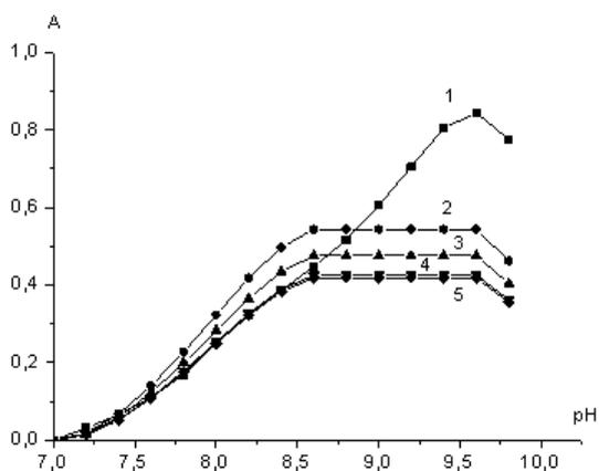
**Figure 3.** Relationships: 1 – total light absorbance of the mixture according- pH at  $\lambda = 555$  nm; 2,3,4,5 – restored light absorbance at  $\lambda = 555$  nm after one, three, fifteen and twenty iterations.
