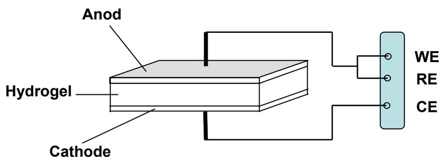
**Figure 3.** Schematics of the ultra thin galvanic cell setups used for testing of Al in hydrogel electrolytes (Anode: metallic Al; Cathode: graphite or MnO<sub>2</sub>; Hydrogel: acrylic polymer; WE – working, RE – reference, and CE – counter electrodes)
