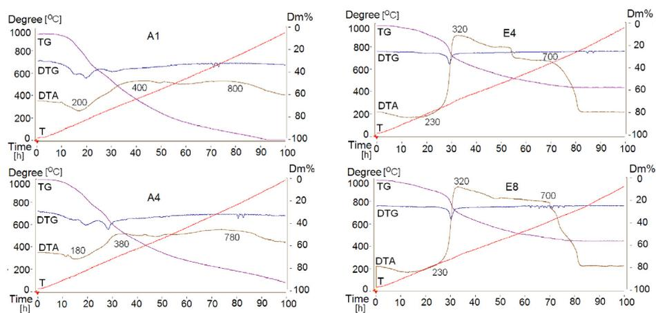
**Figure 1.** The thermal analysis of the dried gels.
