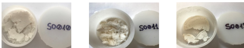
Figure 5. Macroscopic aspect of the lyophilized samples obtained with different gelatin grades (exp. no. SO010 – G \approx 175 Bloom; exp. no. SO011 – G \approx 300 Bloom; exp. no. SO012 – G 80-120 Bloom).
