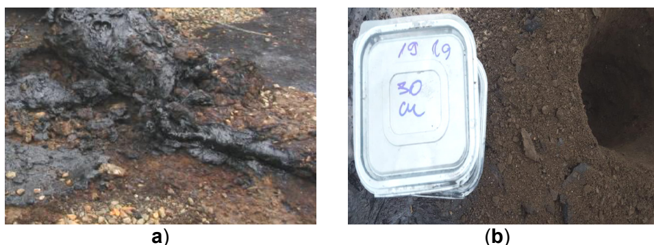
Figure 9. Acid tar, (a) sampling area; (b) acid tar sample analysis, evaluation and validation of treatability test results by performing leaching tests.
