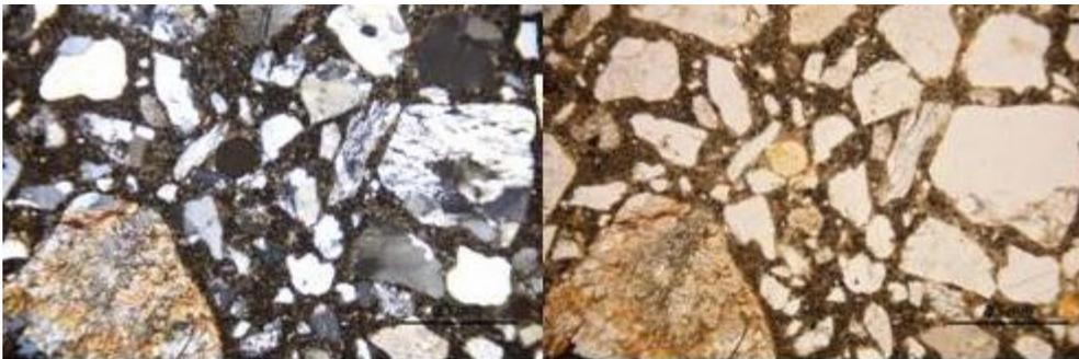
**Figure 7.** Textural aspects of D10 samples, showing a very fine crystallized matrix having rounded pores infilled with iron hydroxides. (Left N+, right NII)
