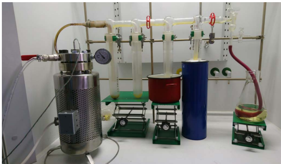
Figure 14. Schematic design of batch reactor used for experimental work in Romania
