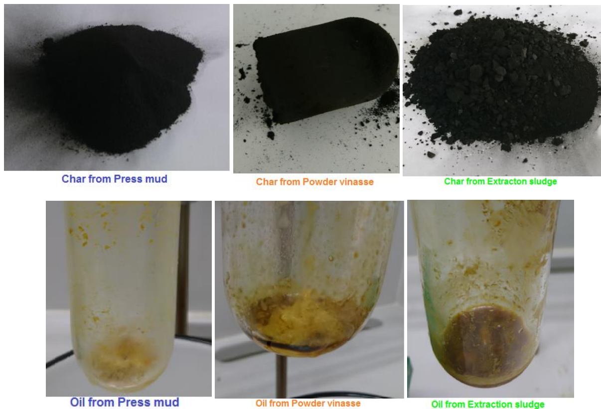
Figure 17. Bio-char and bio-oil from conventional pyrolysis of biomass waste from Bioethanol process
