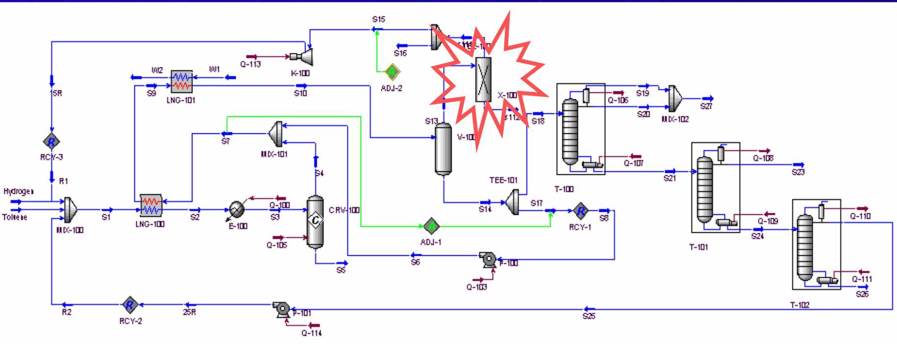
The retrofit alternative design for the HDA process flow sheet<sup>2</sup>
