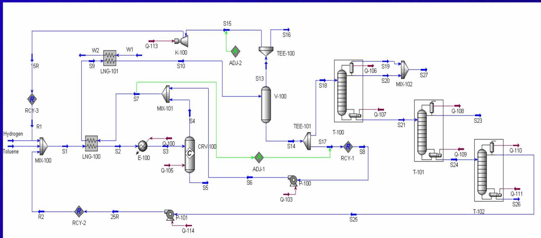
**Hydrogen reacts with Toluene to produce Benzene. Methane is present as impurity and Biphenyl is produced as a by-product**
