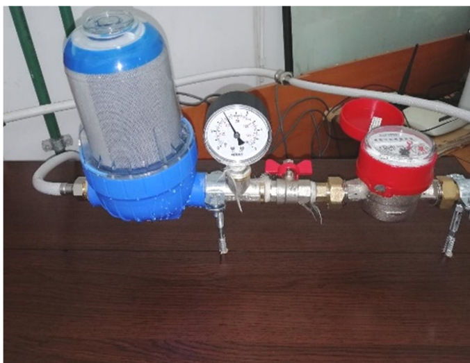
Figure 6. Filter testing on the experimental stand
