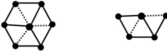
Figure 4. The dotted edges which need to be deleted from a full and a half hexagons.
