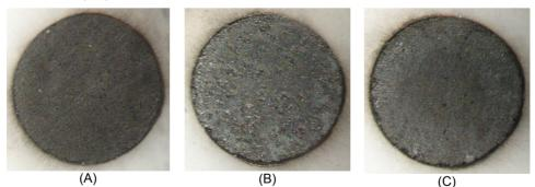
**Figure 5.** Microscopic images of SG/Pb II: the unmodified SG surface (A), after depositing a *approx.* 2 μm PbO<sub>2</sub> layer on the surface (B) and after the completion of the measurements in the 0.2 M vanadium in 2 M H<sub>2</sub>SO<sub>4</sub> solution (C).
