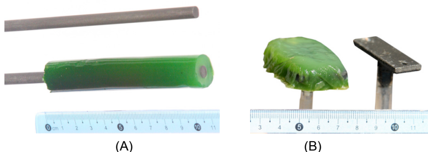
Figure 6. Image of the immobilized Synechocystis cathode and the control cathode (A) for two-chamber (B) for membraneless MFC.
