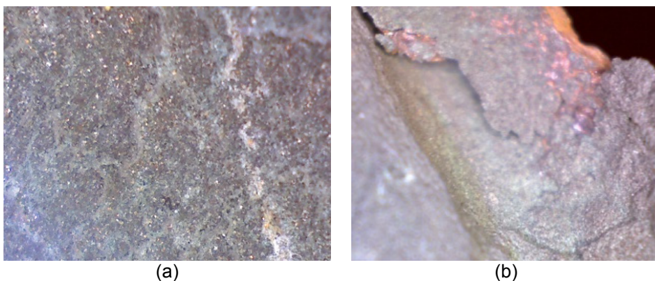
Fig. 1. Microscopic observation of patina on bronze screw from Matthias Rex statuery group: (a), (b) X100.
