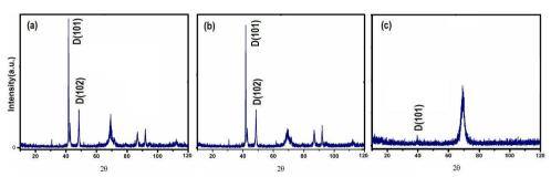
**Fig. 4**. X-Ray diffraction of nano crystalline diamond grown at different substrate temperature (a):550°C; (b):600°C; (c):650°C.
