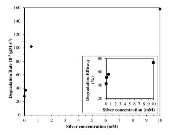
**Figure 5.** The dependence of the silver concentration (in the impregnation step) on the observed degradation rate and degradation efficiency (inserted figure)
