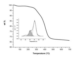
**Figure 2**. TGA thermogram of Laponite Blue with deconvolution of its derivative curve (inset)
