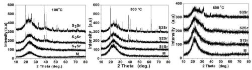
Figure 2. XRD patterns after treatments at different temperatures.
