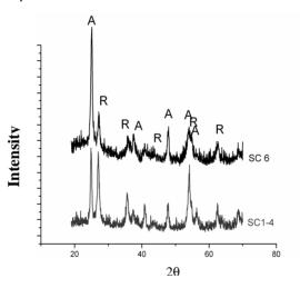
**Figure 1.** X-ray diffraction patterns of the TiO<sub>2</sub> nanopowders. **A** and **R** denote the anatase and rutile phases.
