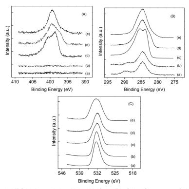
**Figure 3.** XPS high-resolution N 1s (A), C 1s (B), O 1s (C) spectra of glass (a), glass immersed in SBF (b), tetracycline (c), glass with tetracycline (d), and of glass after 96 hours immersion in SBF for tetracycline release (e).
