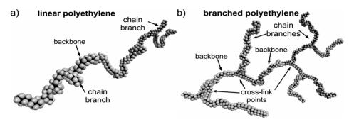
**Figure 1.** Schematic representation of a) liner b) branched polyethylene.
