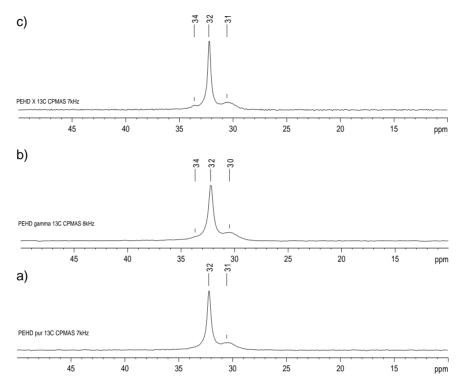
**Figure 4.** CP/MAS <sup>13</sup>C NMR spectra of a) pure; b) gamma irradiated and c) X-ray irradiated high-density polyethylene.
