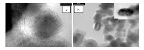
**Figure 3.** TEM micrographs in high resolution mode obtained from the TiO<sub>2</sub> nanopowders: SC 1-4 (a) and SC 6 (b).
