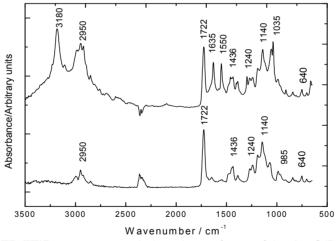
**Figure 1.** ATR FTIR spectra recorded on the surfaces of the Ag<sub>2</sub>O/PMMA before (upper) and after collagen electrodeposition (lower).
