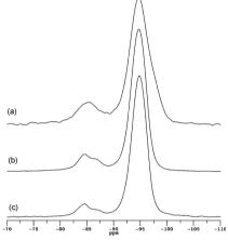
**Figure 5.** <sup>29</sup>Si CP-MAS spectra, recorded at a MAS frequency of 6 kHz, of (a) Laponite RD, (b) Laponite-2C<sub>18</sub>, (c) Laponite Blue
