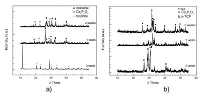
**Figure 2.** XRD patterns of the samples after different aging time periods a) not heat treated b) heat treated at 600 °C
