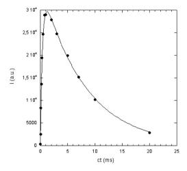
**Figure 8.** Fitting of the CP dynamics curve of the  $^{29}$ Si signal at -86.5 ppm of Laponite-2C<sub>18</sub>. On the *x* and *y* axes contact time values and signal areas are reported, respectively
