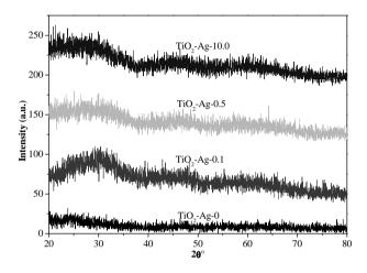
Figure 1. XRD patterns of TiO<sub>2</sub>-Ag photocatalysts
