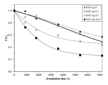
Figure 4. Photocatalytic decay curves of salicylic acid on TiO<sub>2</sub>-Ag catalysts
