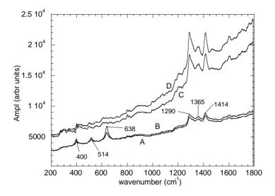
**Figure 3** The Raman spectra of doped and non doped membranes. Curve A, membrane with 20% TiO<sub>2</sub> before irradiation; Curve B, membrane with 20% TiO<sub>2</sub> after 4 hours irradiation UV; Curve C, non doped membrane after 4 hours irradiation UV; Curve D, non doped membrane before irradiation
