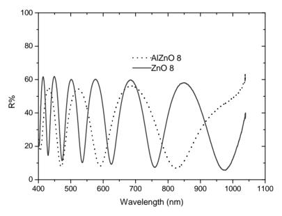
**Figure 4.** Optical reflectance spectra of undoped and Al doped ZnO thin film, both grown under the same conditions (d=8cm).
