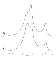
**Figure 9.** 20-45 ppm region of the <sup>13</sup>C CP-MAS spectra of (a) Laponite-2C<sub>18</sub> and (b) Laponite Blue, recorded at a MAS frequency of 6 kHz
