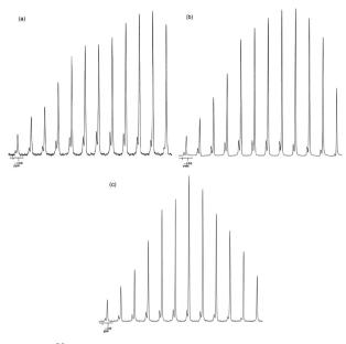
**Figure 7.** Selection of <sup>29</sup>Si CP-MAS spectra of (a) Laponite RD, (b) Laponite-2C<sub>18</sub>, (c) Laponite Blue, recorded at a MAS frequency of 6 kHz and at the same contact time values, ranging between 0.1 and 20 ms
