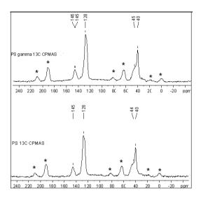
Figure, 2 The CP/MAS <sup>13</sup>C NMR spectra of un-irradiated and gamma irradiated polystyrene
