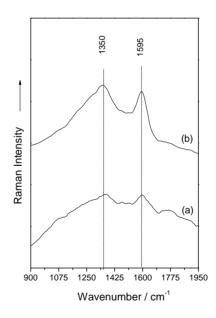
**Figure 4.** Raman spectra of the TiO<sub>2</sub> nanopowders:(a) SC 1-4 and (b) SC 6.
