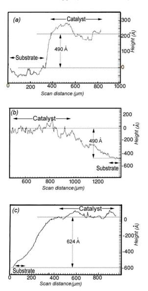
**Fig. 1.** DEKTAK profilometer results show: a) sample A with 21.6nm, b) Sample B with 49nm, and c) sample C with 62.4 nm, for thickness layer.
