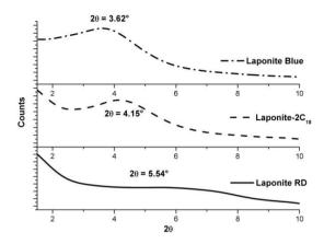
Figure 3. X-Ray diffractograms of Laponite RD, Laponite-2C<sub>18</sub> and Laponite Blue
