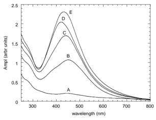
**Figure 2** UV-vis absorption spectra for the doped sample before and after different time intervals of UV irradiation. A). before irradiation; B). after 1 hour irradiation; C). after 2 hours irradiation; D). after 3 hours irradiation; E). after 4 hours irradiation
