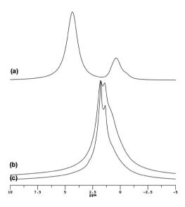
**Figure 6.** <sup>1</sup>H-MAS spectra, recorded at a MAS frequency of 6 kHz, of (a) Laponite RD, (b) Laponite-2C<sub>18</sub>, (c) Laponite Blue
