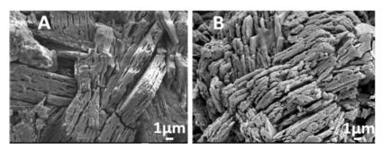
Figure 1. SEM images of bioactive glass before (A) and after (B) tetracycline loading.
