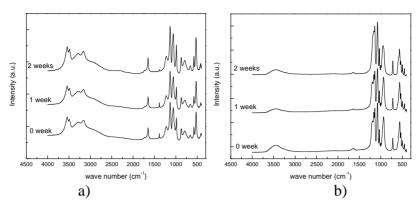
**Figure 5.** FT-IR spectra of the samples washed after different aging time periods a) not heat treated b) heat treated at 600 ℃
