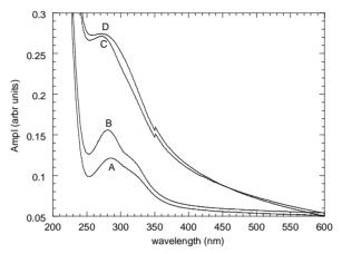
**Figure 1** The UV-vis absorption spectra of doped and non doped membranes: Curve A the non doped membrane after 4 hours UV irradiation; Curve B the non doped membrane before irradiation; Curve C membrane with 10% TiO<sub>2</sub> before irradiation; Curve D membrane with 10% TiO<sub>2</sub> after 4 hours UV irradiation.
