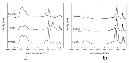
**Figure 4.** FT-IR spectra of the samples after different aging time periods a) not heat treated b) heat treated at 600°C
