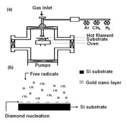
**Figure 1.** Generalized schematic HFCVD system (a) and the growth process in a diamond CVD reactor (b).
