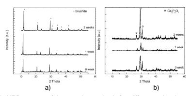
**Figure 3.** XRD patterns of the samples washed after different aging time periods a) not heat treated b) heat treated at 600 ℃
