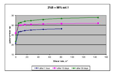
**Figure 5.** Dependence  $\tau = f(\dot{\gamma})$  for sample PC<sub>2</sub> (t=32°C)
