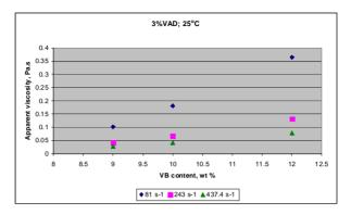
Figure 7. The apparent viscosity vs. the VB concentration
