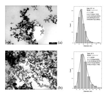
**Figure 2.** TEM micrographs of the TiO<sub>2</sub> nanopowders and the corresponding particle size distributions:(a) SC 1-4 and (b) SC 6.
