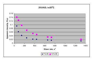
Figure 8. The apparent viscosity vs. shear rate
