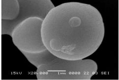
Figure 1. SEM images of the spray dried sample
