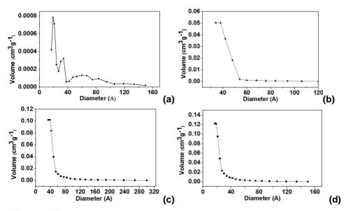
**Figure 4.** Textural pore size distribution of the prepared sample, obtained from BJH analysis of nitrogen desorption branch: (a) M, (b) S1Sr, (c) S2Sr and (d) S3Sr. 196
