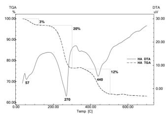
Figure 1. DTA and TG curves of as-prepared sample
