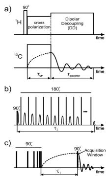
**Figure 3.** a) <sup>1</sup>H -<sup>13</sup>C cross-polarization; b) CPMG and c) saturation recovery pulse sequences.
