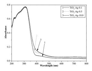
Figure 3. The DRS spectra of selected silver containing titania aerogels
