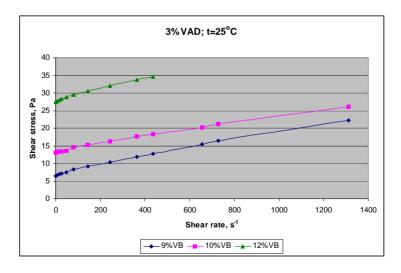
**Figure 6.** Dependence  $\tau = f(\dot{\gamma})$  for PA<sub>3-9</sub>, PA<sub>3-10</sub> and PA<sub>3-12</sub>
