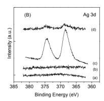
Figure 4. XPS N1s (A) and Ag 3d (B) high resolution spectra of (a) PMMA acrylic cement, (b) PMMA/collagen cement, (c) Ag<sub>2</sub>O/PMMA cement and (d) Ag<sub>2</sub>O/PMMA/ collagen.
