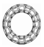
Figure 1. The Zig-zag Polyhex Nanotube.
