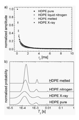
**Figure 5.** a) The CPMG echoes decays; b) the corresponding  $T_2$  distributions for the pure and aged in liquid nitrogen, melted and X-ray irradiated HDPE.
