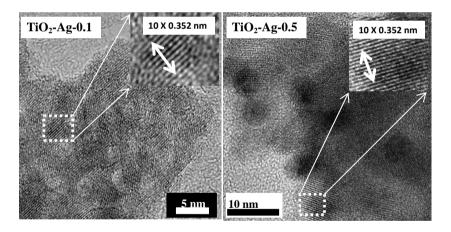
Figure 2. HRTEM micrographs of samples TiO<sub>2</sub>-Ag-0.1 and TiO<sub>2</sub>-Ag-0.5
