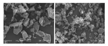
Figure 4. SEM micrograph of (left) Laponite RD and (right) Laponite Blue
