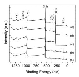
**Figure 2.** XPS survey spectra of glass (a), glass immersed in SBF (b), tetracycline (c), and glass with tetracycline (d) and of glass after 96 hr immersion in SBF for tetracycline release (e).
