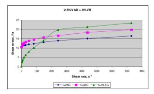
**Figure 1.** Dependence  $\tau = f(\dot{\gamma})$  for PA<sub>2.5-8</sub> at different temperatures
