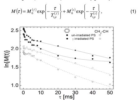
**Figure. 3** Logarithmic plots of  $^{13}$ C resonance intensities corresponding to aromatic (filled symbols) and methylene-methine (open symbols) functional groups function of spin-lock time  $\tau$  for un-irradiated (squares) and gamma irradiated polystyrene (circles).
