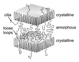
Figure 2. Schematic representation of high density polyethylene morphology.
