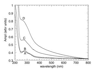
**Figure 2** The UV-vis absorption spectra for the non doped membrane and membranes with different content of TiO<sub>2</sub>, before irradiation. Curve A, the non doped membrane; Curve B, with 1% TiO<sub>2</sub>; Curve C, with 10% TiO<sub>2</sub>; Curve D, with 20% TiO<sub>2</sub>
