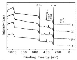
**Figure 3**. XPS survey spectra of (a) PMMA acrylic cement, (b) PMMA cement after collagen electrodeposition, (c) Ag<sub>2</sub>O/PMMA acrylic cement and (d) Ag<sub>2</sub>O/PMMA after collagen electrodeposition.
