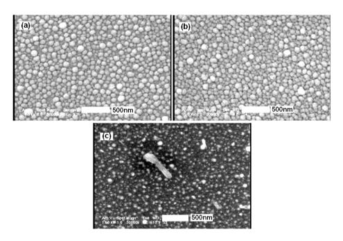
**Fig. 3.** SEM images of nanocrystalline diamond NCD grown at different substrate temperature (a): 550℃, (b):600℃, (c):650℃.
