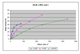
**Figure 3.** Dependence  $\tau = f(\dot{\gamma})$  for sample PC<sub>5</sub>
