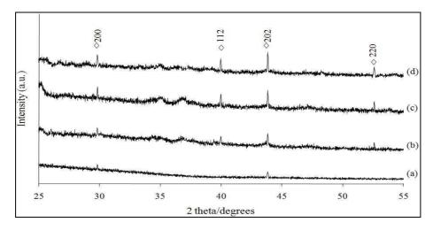
Figure 1. X-ray diffraction patterns for FeS thin films deposited at various bath temperatures. (a) 50 ℃ (b) 60 ℃ (c) 70 ℃ (d) 80 ℃
