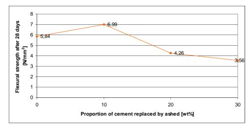
Figure 6. Flexural strength variation in function of proportion of cement replaced by ash.
