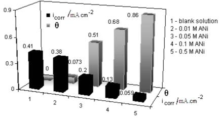
**Figure 2.** Variation of the corrosion current and the degree of coverage with the concentration of aniline for the carbon steel corroded in 0.5 M H<sub>2</sub>SO<sub>4</sub>, at room temperature.
