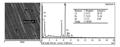
Figure 6. SEM/EDS analysis of the 304L stainless steel sample
