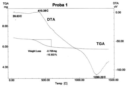
Figure 3. - Thermal behaviour of the ash
