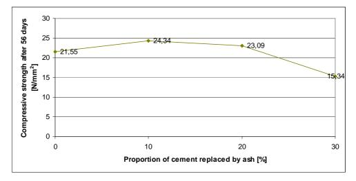
Figure 9. Compressive strength variations in function of proportion of cement replaced by ash
