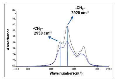
Figure 1. FTIR spectrum of TPH
