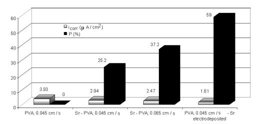
CORROSION BEHAVIOR OF STAINLESS STEEL COATED WITH POLY(VINYL ALCOHOL) FILM ...
