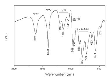
**Figure 1.** FT-IR spectrum of {Mo<sub>132</sub>-U<sup>IV</sup>} cluster.
