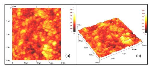
Figure 5. Atomic force microscopy images for FeS thin films deposited at 80 ℃ (a) 2-dimensional (b) 3-dimensional
