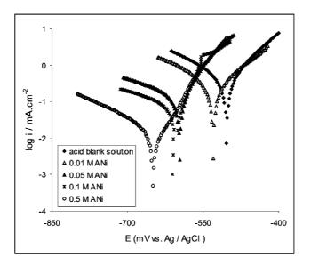
Figure 1. Tafel diagram of carbon steel corroded in  $0.5 \text{ M H}_2\text{SO}_4$  solutions in absence and in presence of ANi inhibitor.
