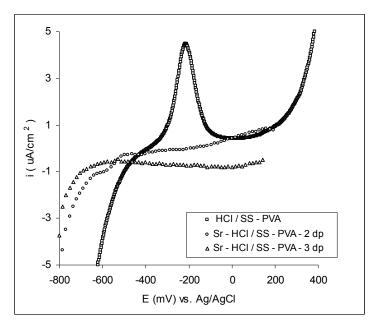
Figure 1. The polarization curves of the modified stainless steel surface with PVA film in 0.1 M HCl solution in absence and in presence of strontium ranelate (potential scan rate, 100 mV / s)
