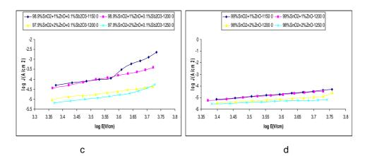
Figure 1. Current density with respect to the applied electrical field for different ZnO and Sb<sub>2</sub>O<sub>3</sub> concentrations
