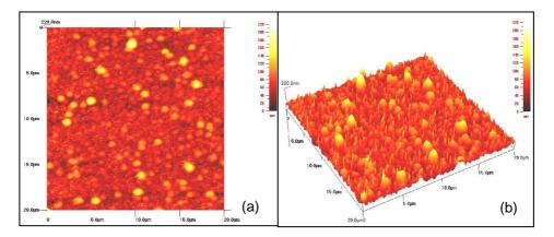
Figure 3. Atomic force microscopy images for FeS thin films deposited at 60 ℃ (a) 2-dimensional (b) 3-dimensional
