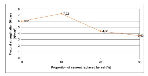
Figure 8. Flexural strength variation in function of proportion of cement replaced by ash.
