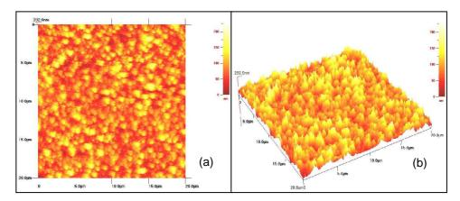
Figure 4. Atomic force microscopy images for FeS thin films deposited at 70 ℃ (a) 2-dimensional (b) 3-dimensional
