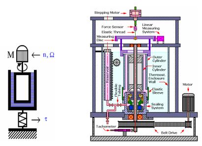
Figure 1 a,b. The Couette modified rheometer.
