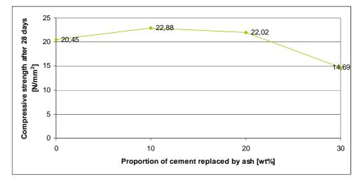
Figure 7. Compressive strength variation in function of proportion of cement replaced by ash.
