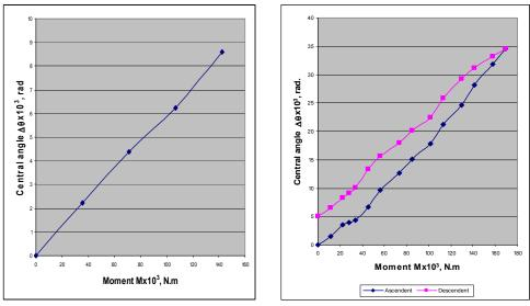
**Figure 4a.** Calibration chart  $\Delta \theta = f(M)$ .
