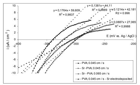
**Figure 4.** Polarization resistance (R<sub>p</sub>) of the stainless steel surfaces modified with PVA and Sr-PVA films, corroded in physiological serum solution.
