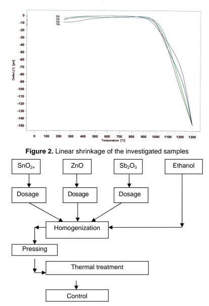
Figure 3. The schematic flux for obtaining the ceramics
