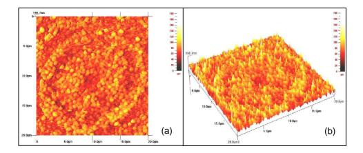
Figure 2. Atomic force microscopy images for FeS thin films deposited at 50 ℃ (a) 2-dimensional (b) 3-dimensional
