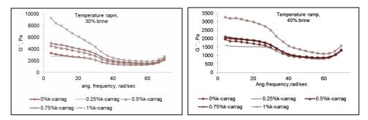
Figure 5. Loss modulus (G``) variation with temperature ramping.
