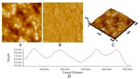
**Fig. 9**. Collagen with doxorubicin film on glass: A) 2D – topography; B) phase image; C) 3D-topography; D) profile of the cross section along the arrow în Fig. 9A. Scanned area: 1 μm x 1 μm.
