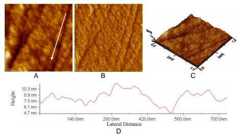
Fig. 5. Fluorouracil film on glass: A) 2D – topography; B) phase image;C) 3D-topography; D) profile of the cross section along the arrow in Fig. 5A. Scanned area: 1 μm x 1 μm.
