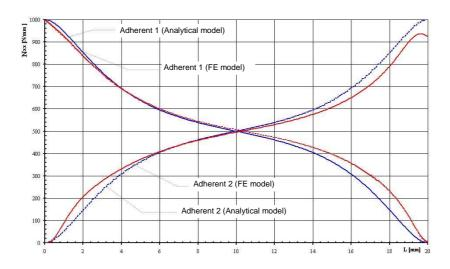
Figure 4. Load transfer in an AU 2024 T3-AV 119-VE ±45° assembly.
