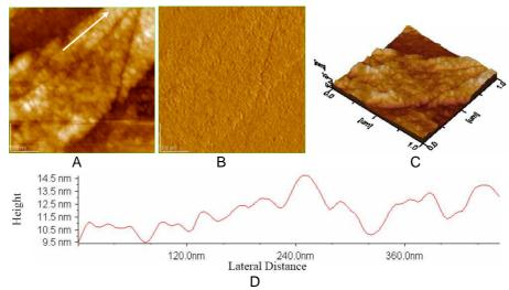
**Fig. 8.** Collagen with 5-fluorouracil film on glass: A) 2D – topography; B) phase image; C) 3D-topography; D) profile of the cross section along the arrow in Fig. 8A. Scanned area: 1 μm x 1 μm.
