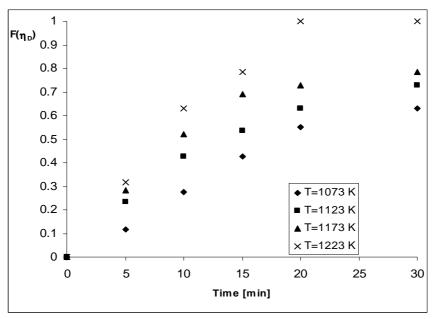
Fig. 5.  $F(\eta_D)$ -time dependence for the unreacted shrinking core model for granules with  $d_p$  =0.063 mm.
