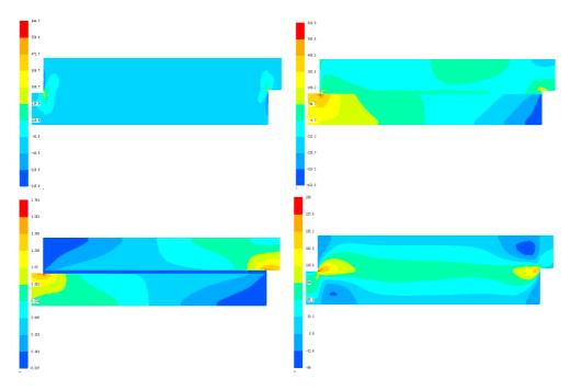
Figure 5. Stress distribution in double-lap bonded joint
