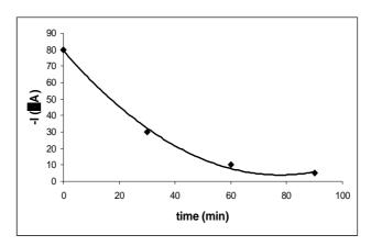
**Figure 5.** The variation of the reduction peak intensity at -0.9 V/Ag/AgCI,KCI, for  $10^{-3} \text{ M 4-NP}$  in  $0.2 \text{ N H}_2\text{SO}_4$ , on Ni (experimental set-up A); i:20 mA cm<sup>-2</sup>; WE: nickel; RE: Ag/AgCI,KCI; CE: Pt.
