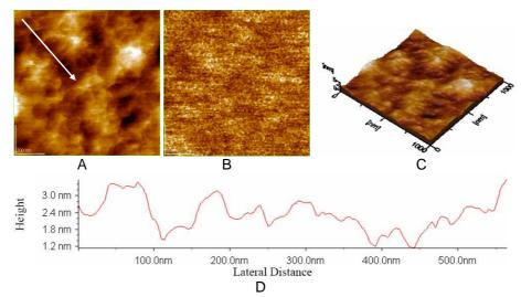
**Fig. 4**. Collagen film on glass, zone 3: A) 2D – topography B) phase image C) 3D-topography, D) profile of the cross section along the arrow in Fig. 4A. Scanned area: 1 μm x 1 μm.
