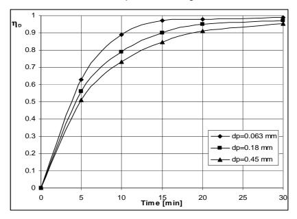
Fig. 2. Particles sizes influence over the decomposition degree of PCC CaCO $_3$  at  $T_c$ =1173 K.
