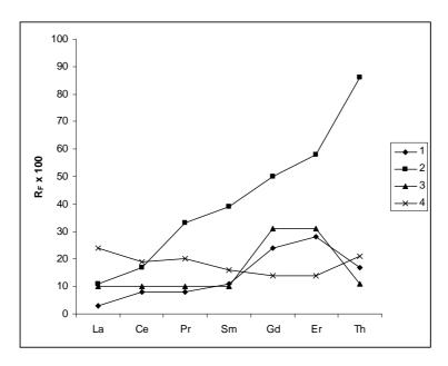
**Fig. 1 -** Retention factors of metal ions for various stationary phases Stationary phase: 1 – silica gel H; 2 – silica gel H impregnated with 2.5M  $NH_4NO_3$ ;3 –silica gel H - Zr(IV) silicate mixture;
