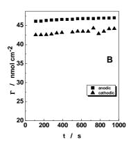
**Figure 1.** (A) Cyclic voltammograms of graphite electrode (---) and of compound **2** adsorbed on graphite (—). (B) Time dependence of surface coverage for compound **2** adsorbed on graphite.
