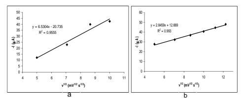
Figure 4. The variation of current with the square root of the scan rate for: (a)  $10^{-3}$  M 4-NP and (b)  $4.5 \times 10^{-4}$  M 2, 6-DNP solutions in in 0.2N H<sub>2</sub>SO<sub>4</sub>; WE: GC; RE: Ag/AgCl,KCl; CE: Pt; v : 50mV s<sup>-1</sup>; s:  $10 \mu$ A V<sup>-1</sup>.
