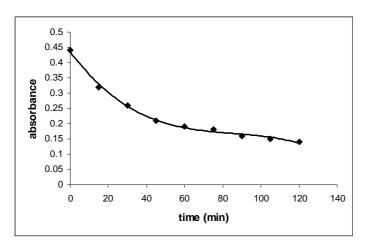
**Figure 7**. Spectrophotometric control of electrochemical reduction process for  $10^{-2}$  M 4-NP in 0.2 N H<sub>2</sub>SO<sub>4</sub> on graphite cathode (B);  $\lambda_{max} = 318$  nm; log  $\varepsilon = 3.87$ .
