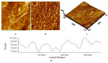
**Fig. 1.** Collagen film on glass, zone 1. A) 2D – topography B) phase image C) 3D-topography, D) profile of the cross section along the arrow in Fig. 1A. Scanned area: 1 μm x 1 μm.
