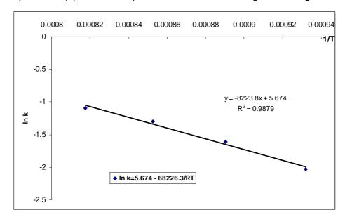
**Fig. 7.** In k versus 1/T variation for PCC granules with  $d_p$ =0.063 mm.
