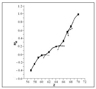
**Fig. 3** - Dependence of  $R_{\rm M}^*$  on Z for the investigated lanthanides. Stationary phase: silica gel H impregnated with 2.5 M NH<sub>4</sub>NO<sub>3</sub>; *Mobile phase*: MEK-THF (6.8 : 3.2, v/v)- 0.4 M HDEHDTP
