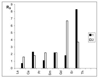
**Fig. 2 -** Resolution of separation of Th(IV) and Ln(III) on silica gel H impregnated with 2.5M NH<sub>4</sub>NO<sub>3</sub>; *Mobile phase*: MEK – THF (6.8 : 3.2 , v/v)– 0.4 M HDEHDTP mixture; 1 – simple elution; 2 – double elution.
