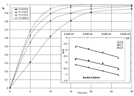
Fig. 3. Temperature influence over the decomposition degree of PCC granules with  $d_{\text{p}} = 0.063 \text{mm}$ .
