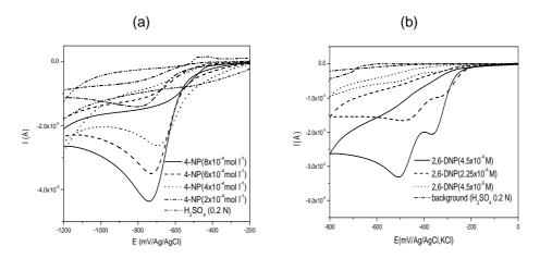
**Figure 1.** Cyclic voltammograms for: (a) 4-NP solutions at different concentrations, in 0.2N  $H_2SO_4$ ; (b) 2,6-DNP solutions at different concentrations, in 0.2N  $H_2SO_4$ ; WE: GC; RE: Ag/AgCI,KCI; CE: Pt; v: 50mV s<sup>-1</sup>; s: 10  $\mu$ A V<sup>-1</sup>.
