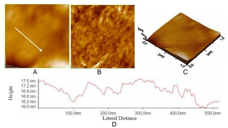
Fig. 3. Collagen film on glass, zone 2: A) 2D – topography B) phase image C) 3D-topography, D) profile of the cross section along the arrow in Fig. 3A. Scanned area: 1  $\mu$ m x 1  $\mu$ m.
