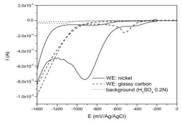
**Figure 2.** Cyclic voltammograms for a (10<sup>-2</sup> M) 4-NP solution in 0.2N H<sub>2</sub>SO<sub>4</sub> WE: GC and Ni; RE: Ag/AgCl,KCl; CE: Pt; v : 50mV s<sup>-1</sup>; s: 100 μA V<sup>-1</sup>.
