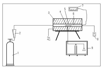
**Fig. 1**. Experimental set-up for PCC calcination 1-Gas cylinder with N₂; 2- Gas flow meter; 3- Electric Furnace; 4- Nacelle with solid sample; 5-Tubular reactor; 6- Thermocouple; 7- Temperature controller; 8- Absorbing vessel for gas; 9- Thermo balance
