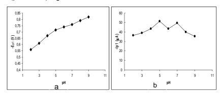
**Figure 3.** The variation of: **(a)** the first reduction peak potential ( $E_{p1}$ ); **(b)** current intensity, with the pH, for a 4.5 x 10<sup>-4</sup> M 2,6-DNP solution in Britton-Robinson buffer at different pH values WE: GC; RE: Ag/AgCl,KCl; CE: Pt; v:50mV s<sup>-1</sup>; s: 10  $\mu$ A V<sup>-1</sup>.
