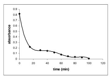
**Figure 8.** Spectrophotometric control of electrochemical reduction process for 4.5 x  $10^{-5}$ M 2,6-DNP in (0.1N) NaCl, on graphite cathode (experimental set-up C).  $\lambda_{max} = 440$  nm; log  $\varepsilon = 3.58$ .
