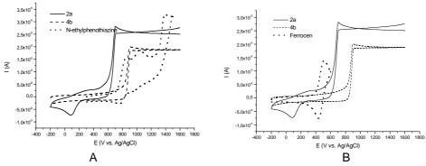
**Figure 2**. Cyclic Voltammograms of: A) **2a, 4b**, N-ethylphenothiazine; B) **2a, 4b**, ferrocen. Experimental conditions: solvent DMF, supporting electrolyte 0.1M LiClO<sub>4</sub>, GC electrode, scan rate v=100 mVsec<sup>-1</sup>
