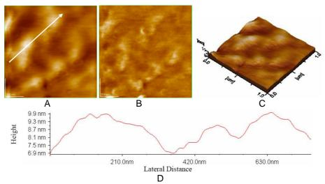
Fig. 7. Lipoic acid film on glass: A) 2D – topography; B) phase image; C) 3D-topography; D) profile of the cross section along the arrow in Fig. 7A. Scanned area: 1  $\mu$ m x 1  $\mu$ m.
