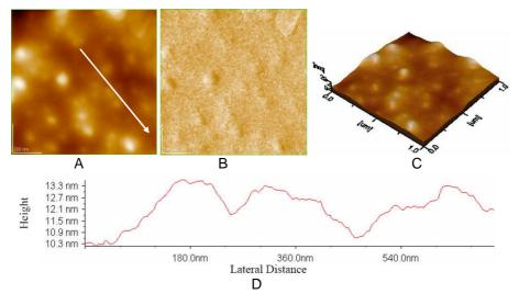
Fig. 6. Doxorubicin film on glass: A) 2D – topography; B) phase image; C) 3D-topography; D) profile of the cross section along the arrow in Fig. 6A. Scanned area: 1  $\mu$ m x 1  $\mu$ m.
