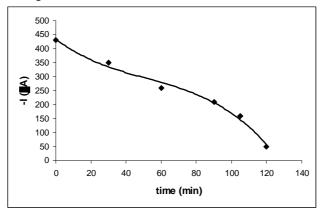
**Figure 6.** The variation of the reduction peak intensity during electrochemical reduction process for 10<sup>-2</sup> M 4-NP in 0.2 N H<sub>2</sub>SO<sub>4</sub>, on graphite cathode (experimental set-up B); i: 20 mA cm<sup>-2</sup>.
