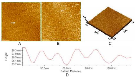
**Fig. 10**. Collagen with lipoic acid film on glass: A) 2D – topography; B) phase image; C) 3D-topography; D) profile of the cross section along the arrow in Fig. 10A. Scanned area: 1  $\mu$ m x 1  $\mu$ m.
