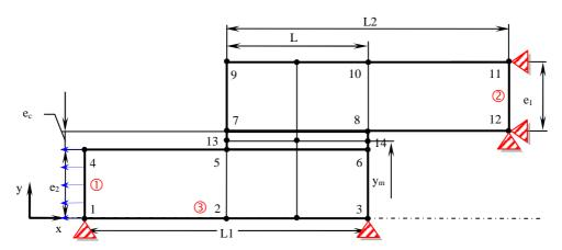
Figure 1. CAD diagram of a double-lap adhesive-bonded joint.
