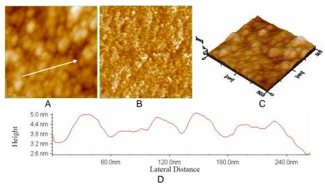
**Fig. 2**. Collagen film on glass, zone 1: A) 2D – topography B) phase image C) 3D-topography, D) profile of the cross section along the arrow in Fig. 2A. Scanned area:  $0.5~\mu m \times 0.5~\mu m$ .
