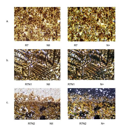
**Figure 5.** Optical microscopy images of the R7 sample obtained after the second crystallization thermal treatment (x90)
