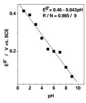
**Figure 3.** pH dependence of the formal potential of DAPht adsorbed on graphite. Experimental conditions: scan rate, 5 mV s<sup>-1</sup>; supporting electrolyte, 0.1 M phosphate buffer.
