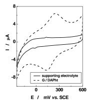
**Figure 2.** Cyclic voltammograms for DAPht adsorbed on spectrographic graphite. Experimental conditions: starting potential, –250 mV vs. SCE; scan rate, 10 mV s<sup>-1</sup>; supporting electrolyte, 0.1 M phosphate buffer (pH 7); surface coverage, see Table 1.
