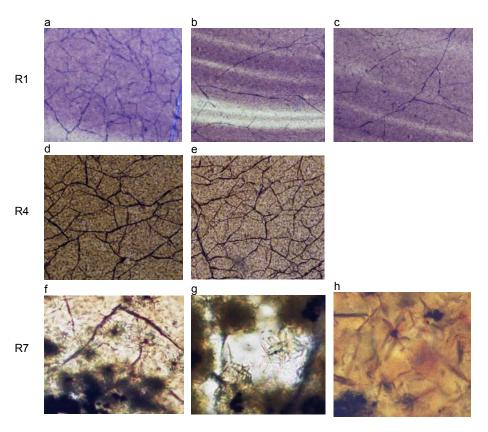
Figure 3. Optical microscopy images of the samples obtained after the first crystallization thermal treatment (x90)
