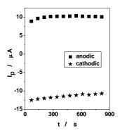
**Figure 4.** Time dependence of the peak current intensity for G/DAPht modified electrodes. Experimental conditions: scan rate, 50 mV s<sup>-1</sup>; potential range, -250 to 600 mV vs. SCE; supporting electrolyte, 0.1M phosphate buffer (pH 7).
