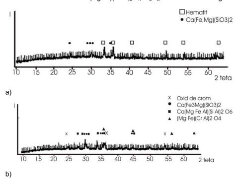
Figure 7. X-ray diffraction pattern for the samples R1N1 (a) şi R1N2 (b)
